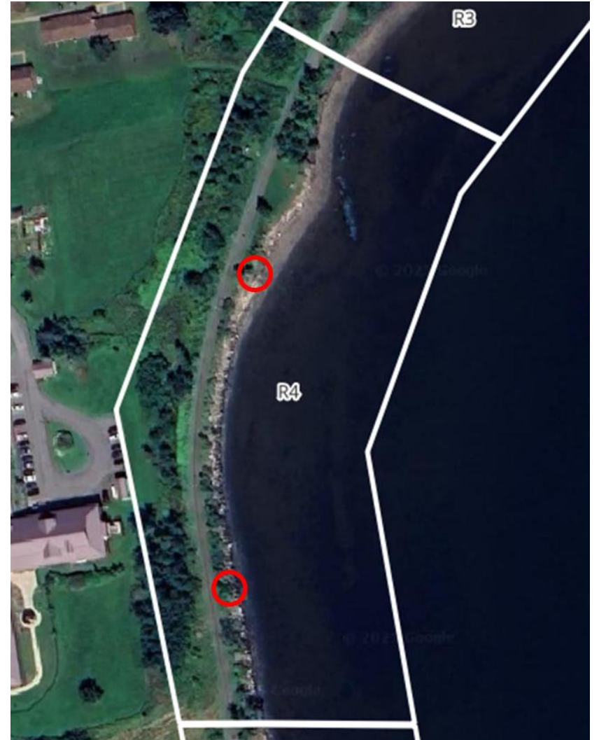
Recommended test pit locations for geotechnical investigation.
